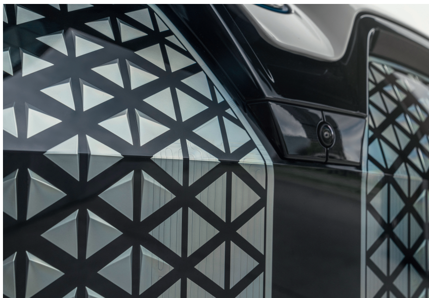
Fig. 1. The striking front panel of the BMW iX is made of the PC Makrolon AG from Covestro. Camera technology, radar functions and other sensors for the driver assistance system are all integrated into the large-scale component. © BMW
